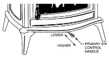
PUSH IN ALL THE WAY (TO RESET CONTROL PLATES), THEN PULL OUT IN INCREMENTS TO DESIRED HEAT OUTPUT SETTING.
